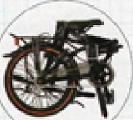
**DETAIL:** Flip two latches and drop the seat post — which doubles as a tire pump — to fold up the Dahon.
